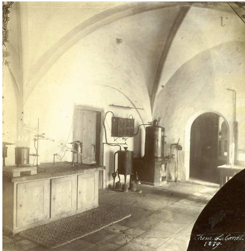
Fig. 4. The laboratory in the former kitchen of the castle in Tübingen as it was in 1879. It was in this room that Miescher had discovered DNA 10 years earlier. The equipment and fixtures available to Miescher at the time would have been very similar, with a large distillation apparatus in the far corner of the room to produce distilled water and several smaller utensils, such as glass alembics and a glass distillation column on the side board. Photography by Paul Sinner, Tübingen.
